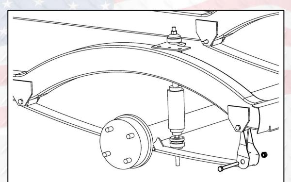
11. Using a 10mm socket and 13mm wrench remove hardware from rear leaf spring mount and front leaf spring mount. Retain hardware.
