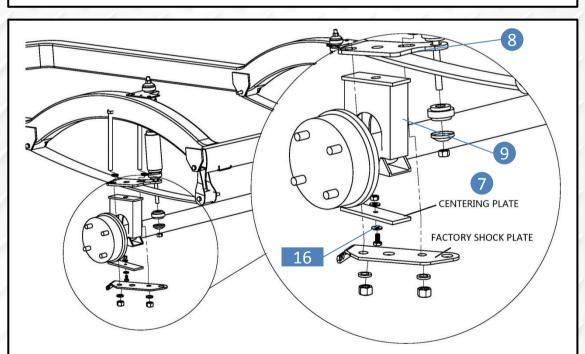
13. Place rear lift block #9 on the axle and under leaf spring. Ensure that top of lift block angles down toward the front of cart. Place rear shock plate #8 over leaf spring and attach shock to it. Attach hardware #16 on centering plate #7 then attach centering plate to factory shock plate. The bolt head and nut will fit into the center hole of the spring perch and factory shock plate to aid in alignment of the riser and mounting plates.
