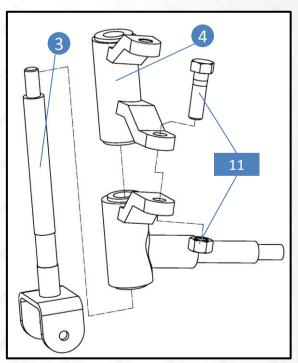
5. Before moving to next step, install spindle riser #4 and factory spindle on supplied kingpin #3 with supplied hardware #11.
