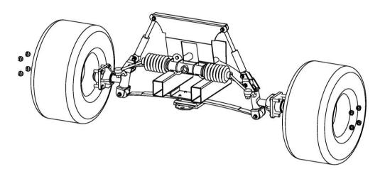
1. Remove lug nuts when cart on ground. Then raise the cart with jack stands under the frame. Remove wheel from the hub. Detach front bumper and retain hardware.
