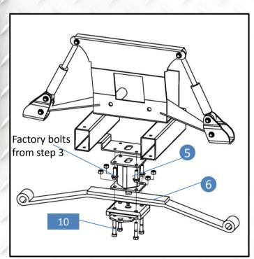
4. Attach retaining plate to front lift block #5 with supplied leaf spring #6 sandwiched in middle, using supplied hardware #10 to secure. Attach lift block assebmly to cart frame using hardware from step 3.
