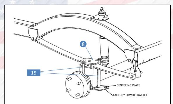
13. Route supplied bolts M12\*180 through shock mounting plate, rear lift block and factory shock plate. Using socket to tighten these four bolts evenly to ensure proper alignment.
