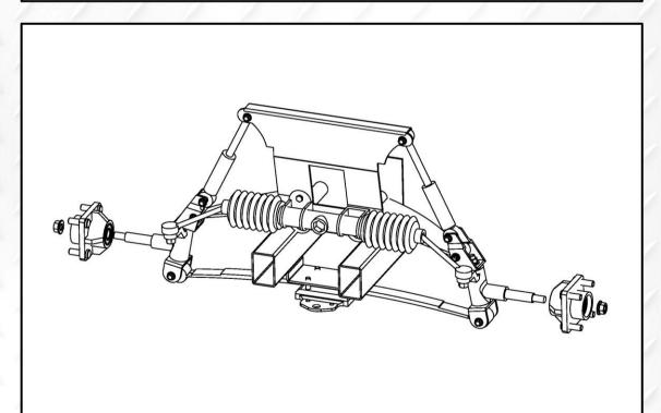
2. Using a 21mm socket remove and retain hub and flange nut. Repeat on passenger side.
