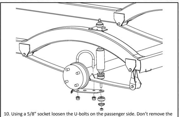
U-bolts. It's important to do one side at a time to avoid motor roll. Loosening but not
