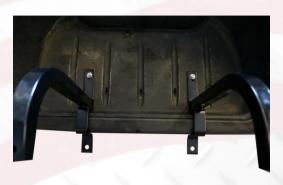
Step 5: Install vertical supports on cart's bagwell area using hardware D-6. You have to enlarge the mounting hole using supplied drill bit. Reattach the access panel cover back to cart using original factory fasteners.
