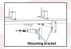
1. Install mounting bracket to footplate using 4 supplied 1/4-1 3/4 bolts, washers and nuts.
