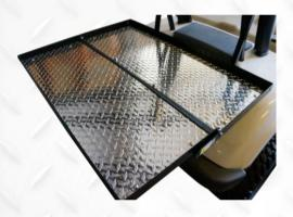
Step 6: Install flipping cargo bed on vertical support and on main bracket using hardware D-2.
