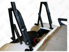
Step 4: Install two rear roof supports on main brackets using hardware D-5
