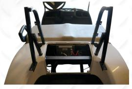
Step 3: Install main bracket on cart using original factory hardware. Tight the bolts from inside the cart.
