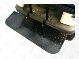
Step 7: Install foot plate on vertical supports using hardware D-4.
