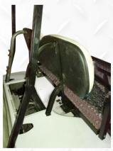
Step 9: Install front back cushion using factory hardware. Install rear seat back cushion on the main bracket using hardware D-3.
