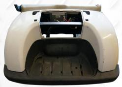
Step 1: Take off canopy / front backrest cushion pad / rear roof support bars (plastic and steel both) / main brackets (with bag holder and basket) / plastic access panel cover.
