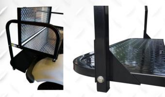
Step 8: Install arm tubes, the bolt points outwards. Use hardware D-1. Use longer bolts on foot plate. Install triangle brackets between arm tube and under footplate.
