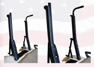
Step 4: Install plastic water drain rear roof support bars on steel rear roof support bars using original factory fasteners.
