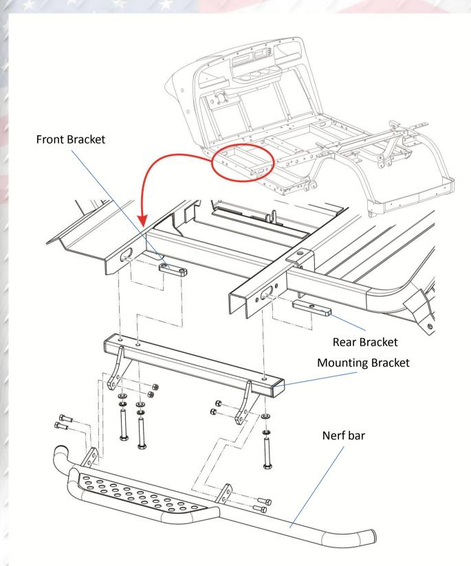
Attach front bracket and rear bracket to cart. Install mounting bracket on front and rear brackets using hardware #2. Install nerf bar to mounting bracket using hardware #1. Repeat on the other side.
